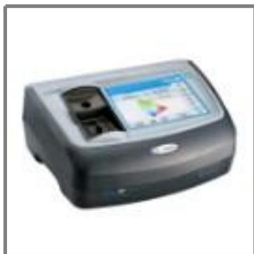
Exact colour calculations which conform to several DIN-ISO-ASTM standards or AOCS Methods are done with only one measurement. Traditional visual colour values like the iodine colour value, Hazen or Gardner are displayed as well as modern colour systems, e.g. CIE-L\*a\*b\* or colour measurements corresponding to European or US pharmacopeia.
