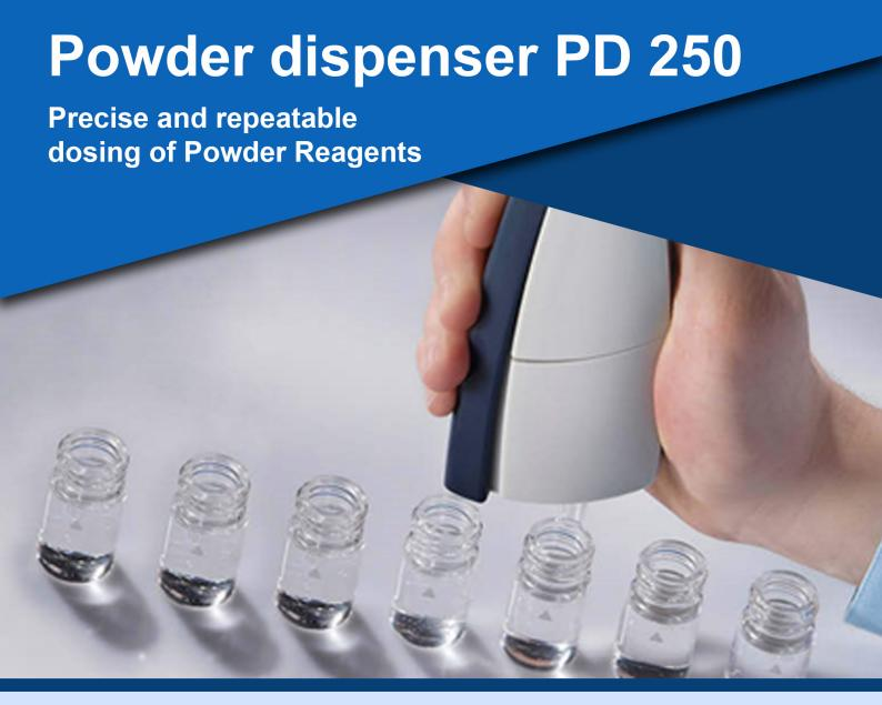
The PD250 is designed for easy and controlled dosage of DPD powder reagents. One click gives the exact amount of reagent required for a 10 ml sample. The PD 250 is the perfect alternative to the Powder Packs for those carrying out a number of tests, saving time while also reducing the amount of packaging waste.
