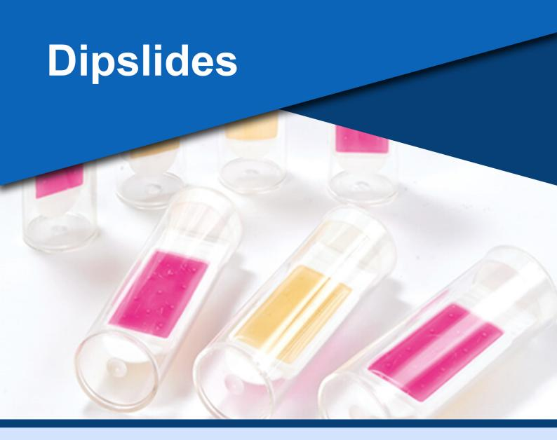
Guidelines to advise on the correct practices to control legionella bacteria in water systems exist world-wide. Suppressing bacteria levels does substantially reduce the possibility of an outbreak of this often fatal disease. Guidelines recommend introducing a monitoring and control program. This program includes the testing of cooling tower waters with dipslides on a regular basis.
